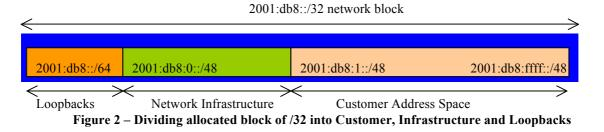
Study the address plan which was handed out as an addendum to this workshop module. Notice how the infrastructure addressing uses the first /48 out of the /32 address block. Notice how we have set a side on /64 out of the infrastructure block for the router loopbacks. ISPs tend to document their addressing plans in flat text files or in spreadsheets – Figure 3 below shows an extract from a typical example (using our addressing scheme here).
